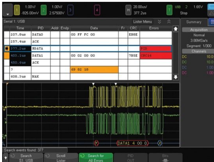
Figure 21. USB 2.0 trigger, decode and "lister" display.
