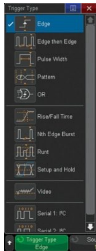
Figure 41. Wide array of advanced parametric trigger modes.
