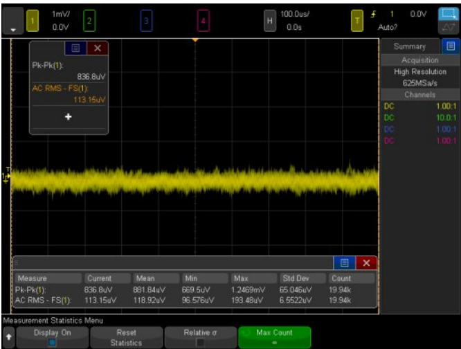
Figure 40. Getting 113 \mu Vrms noise floor at 1 mV/div with the high-resolution mode.
