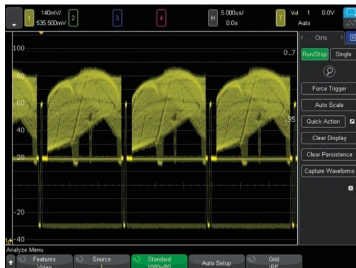
Figure 27. Triggering on 1080p HDTV signal analysis.
