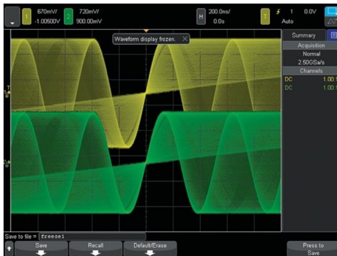
Figure 42. The “freeze screen” feature keeps the intensity-grading information while stopping the waveform acquisition.
