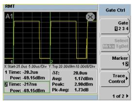
100 MSa/s continuous sampling ensures signal glitches are not missed Time-gated peak, average and peak-to-average ratio power measurements
