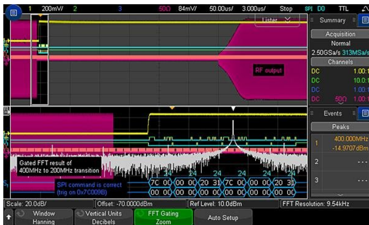
Figure 21. Triggered on a SPI command, the RF signal is still at 400 MHz as indicated in the frequency peak search result lister.
