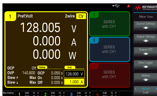
Figure 3: Increase output voltage with E364SNP kit.
