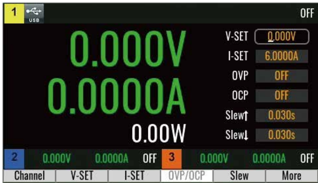
Single-Channel Meter Interface and Quick Setup Interface
